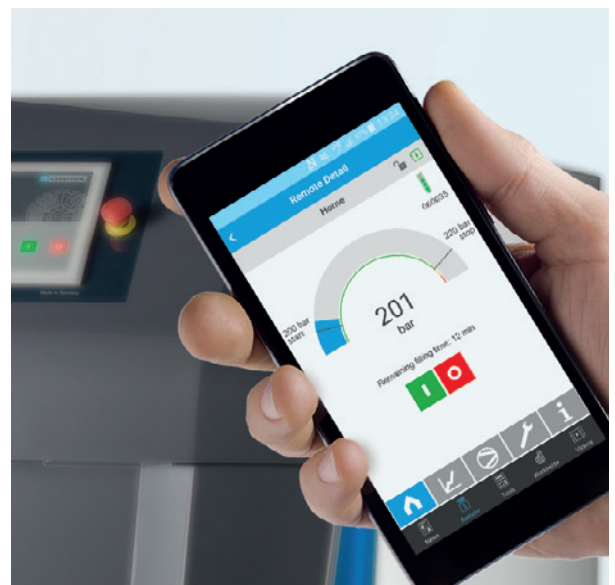
The new B-APP turns your smartphone into a compressor control unit.
